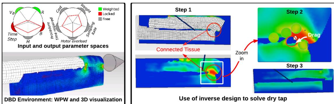
Figure 1. Resolution of a dry tap using the inverse design in DBD
