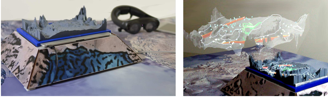
Figure 5.4: (Left image) The physicalization and force-sensing surface are placed on a truncated pyramidal base. The base is situated onto a large fabric poster with contextual NASA satellite imagery around the Filchner-Ronne ice shelf in the Antarctic. The imagery is not to scale with the physicalization. (Right image) Worlds-in-miniature allow the user to view their data at multiple scales. All interactions still take place on the physicalization; when users are focused on the larger world, the physicalization acts as a haptic proxy.
