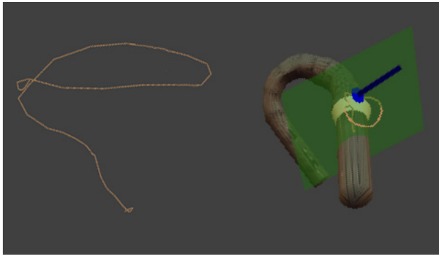
Figure 2. Proper gesture segmentation is required when determining the best-fit plane to project gesture points onto for recognition. The image on the right shows how the user has pulled the pen way from the prop surface after indicating the start of a gesture, causing the best fit plane to be almost perpendicular to the plane that contains the “real” gesture. The image on the left shows the sketch input projected onto the best fit plane and scaled to fit within a square.
