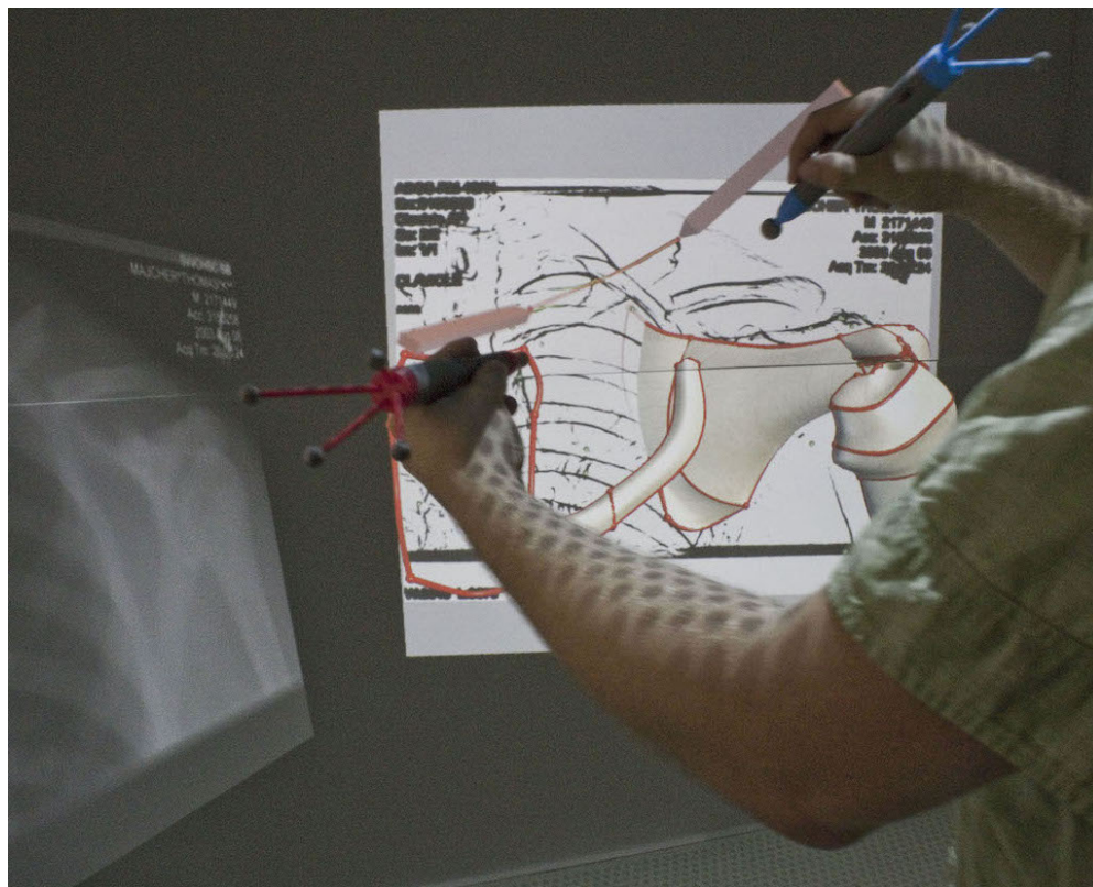
(c) Users place these data images as slides in 3D space and then “Lift-Off” curves to construct 3D models and annotations
