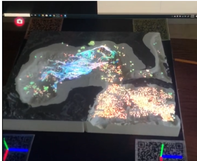
Figure 7.13: An ABR visualization being remotely rendered into a Magic Leap to be viewed with a 3D printed bathymetry.
