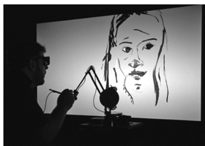
Fig. 2. The Drawing on Air interface with mechanical pen force feedback device. (© 2009 Daniel F. Keefe)
