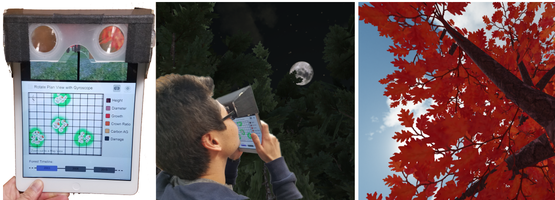
Figure 4.1: Constructing a low-cost, mobile VR device as shown makes it possible to hold the display up to ones eyes and see a stereoscopic 3D visualization and also interact with a linked complementary 2D visualization displayed on the bottom of the screen.
